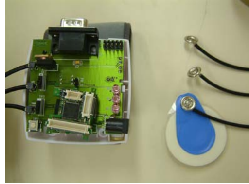
Figure 4.9: (B) The Tyndall-DMS-Mote with three ECG cables attached, positive, negative and ground.
