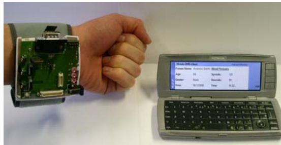
Figure 8.1: An Exposed Tyndall-DMS-Mote prototype and Mobile-DMS-Client (i.e. Jade-Leap agent on a Nokia 9500) displaying blood pressure readings and patient details.
