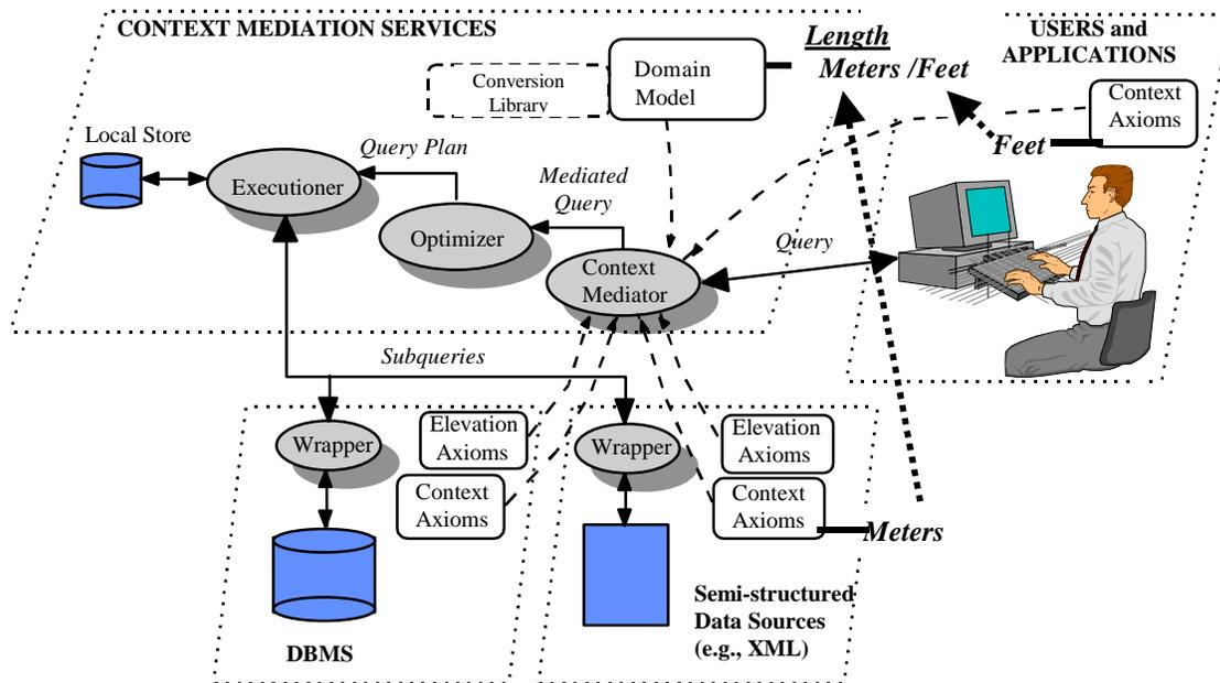
**Figure 4. The Architecture of the Context Interchange System**
