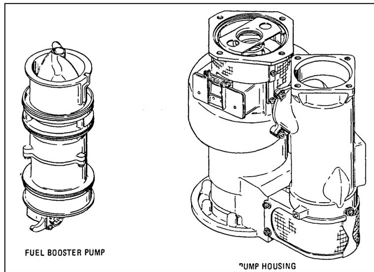
Figure 1: Fuel Booster Pump and Pump Housing
