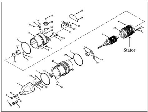
Figure 2: An Illustrative Stator position in the Fuel Booster Pump, Exploded View
